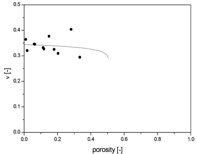
Figure 2 Poisson's ratio porosity dependence for porous ZnO [4].
