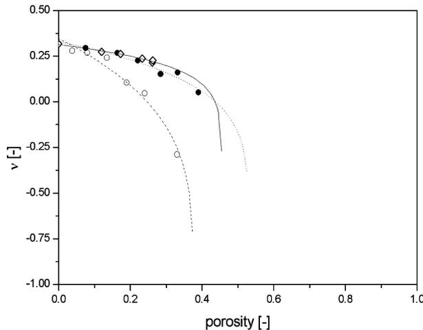
Figure 4 Influence of powder size on Poisson's ratio porosity dependence for porous Th<sub>2</sub>O [8]: (○) 0-2  $\mu\text{m}$ ; (●) 2-4  $\mu\text{m}$ ; (◇) 4-44  $\mu\text{m}$ .
