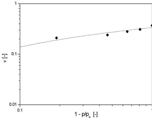
Figure 3 Log-log plot of Poisson's ratio vs.  $1-p/p_c$  for sintered alpha-two titanium aluminide [5] ( $p_c \equiv 0.37$  is tap porosity).
