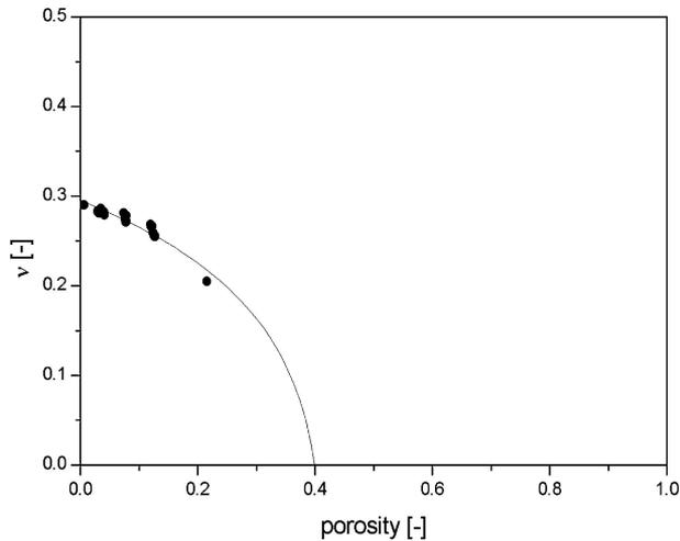
Figure 1 Poisson's ratio porosity dependence for sintered iron [3].
